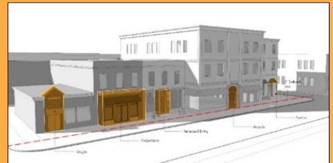
Spacing for first floor entrances
