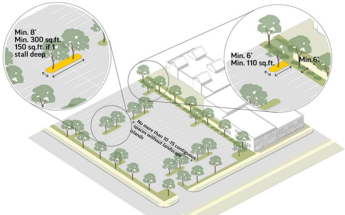
Figure 7-3. Parking lot landscape should be designed to enhance relationships to the streetscape, buffer parking from adjacent areas, and soften large expanses of parking. The standard increase the large the parking area and the more publicly visible the location.
