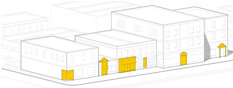
Figure 6-9. Frequent human-scale entry featured relate buildings to streetscapes and public spaces and are more important the closer the building is to the street and the more pedestrian oriented the street or public space that the building fronts on.
