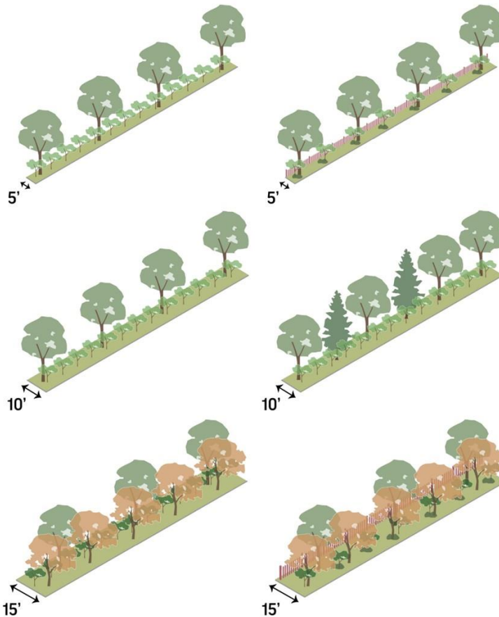
Figure 8-6. Buffers include 3 types based on the degree of intensity to be mitigated, and are based on options that combine space, landscape, and/or structural elements.
