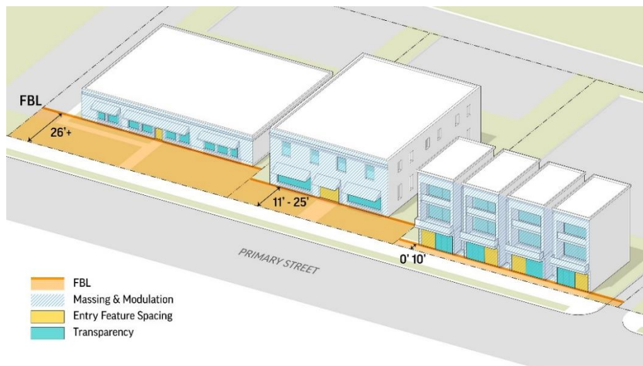
Figure 6-7. Building massing and modulation is determined by the form of the building and details distinguishing different massing elements, the entry location and frequency, extent and location of windows, and use of different complimentary materials.
