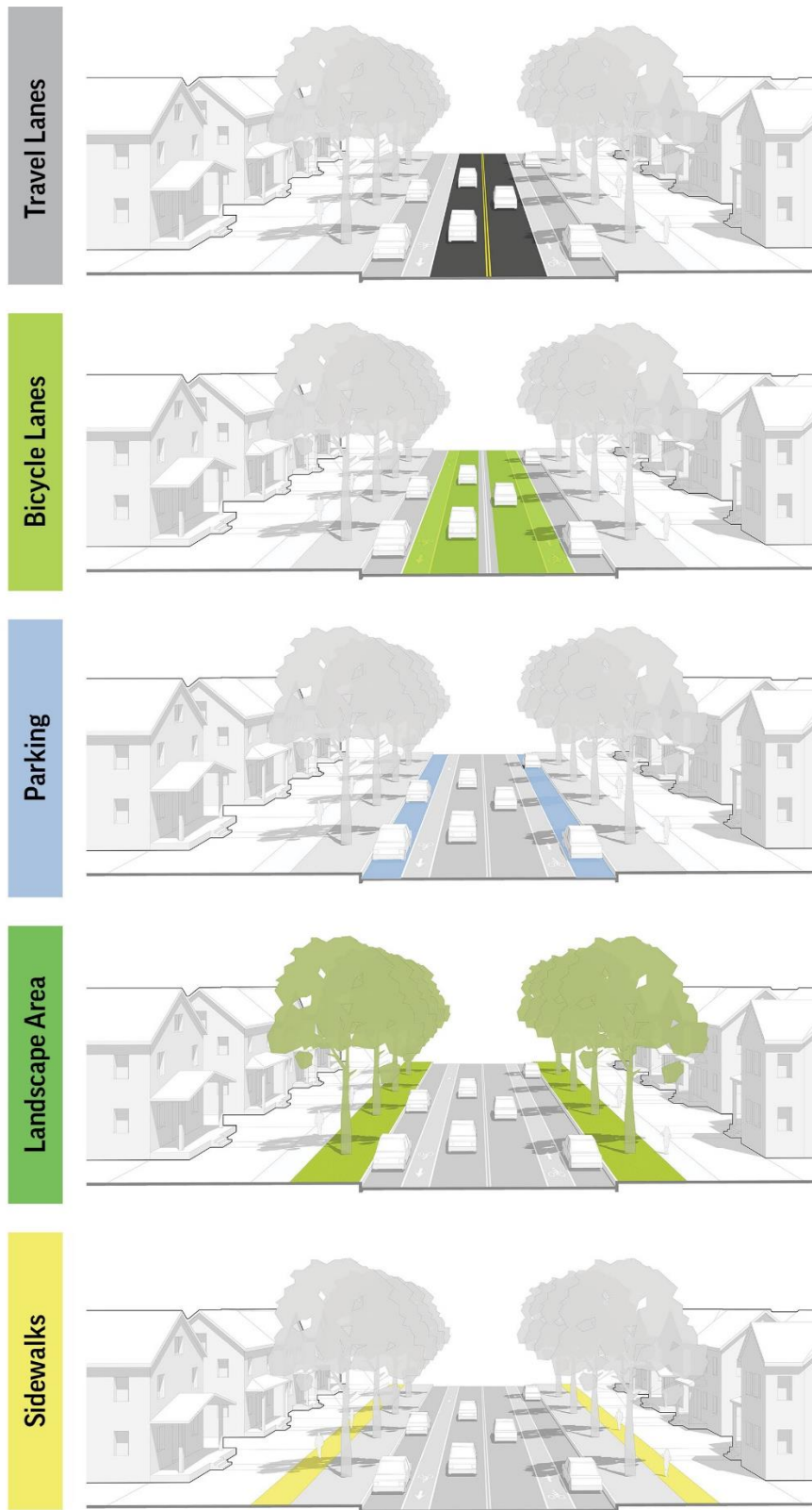
Figure 3-3. Streetscape elements may be adjusted to reflect different priorities for different components of streets in a specific context or to address or to address ROW constraints. Table 3-3 provides a guide for adjusting elements within the requirements of the Street Design Types in Table 3-2.
